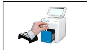
The door opens automatically. Insert the cartridge (Cuvette with Reagent Cap) into the Chamber and close the door. The test starts automatically.
