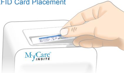
Take the provided RFID card out of the test kit and place it on the RFID card well on top of the Analyser.
